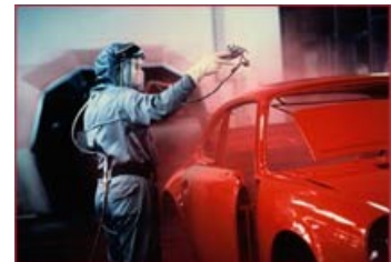
Car body sprayed with cellulose paint for protection and aesthetic purposes
