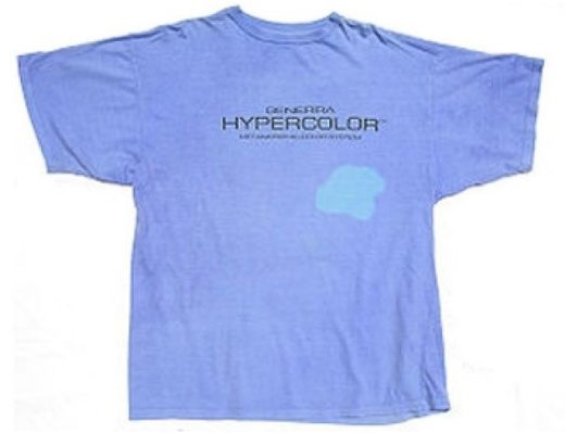
Thermochromic ink on fabrics which changes colour when submitted to heat
